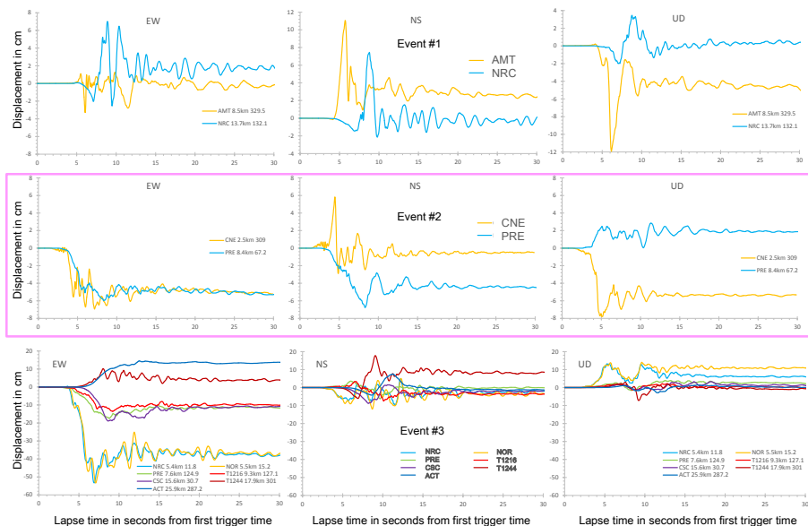
Figure 14. Displacements derived from the double integration of the strong motion for Events #1 to #3
