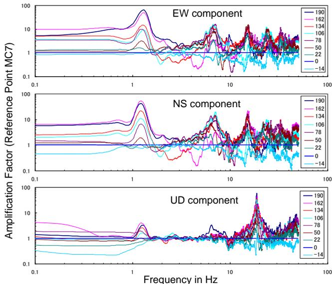
**Figure 8.** Amplification Spectra of AC estimated from Individual Measurement
