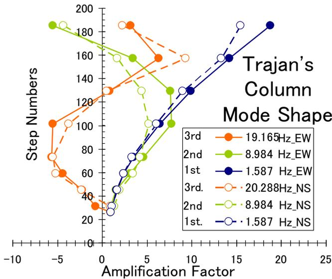
Figure 4. Mode Shape of TC estimated from Simultaneous Measurement
