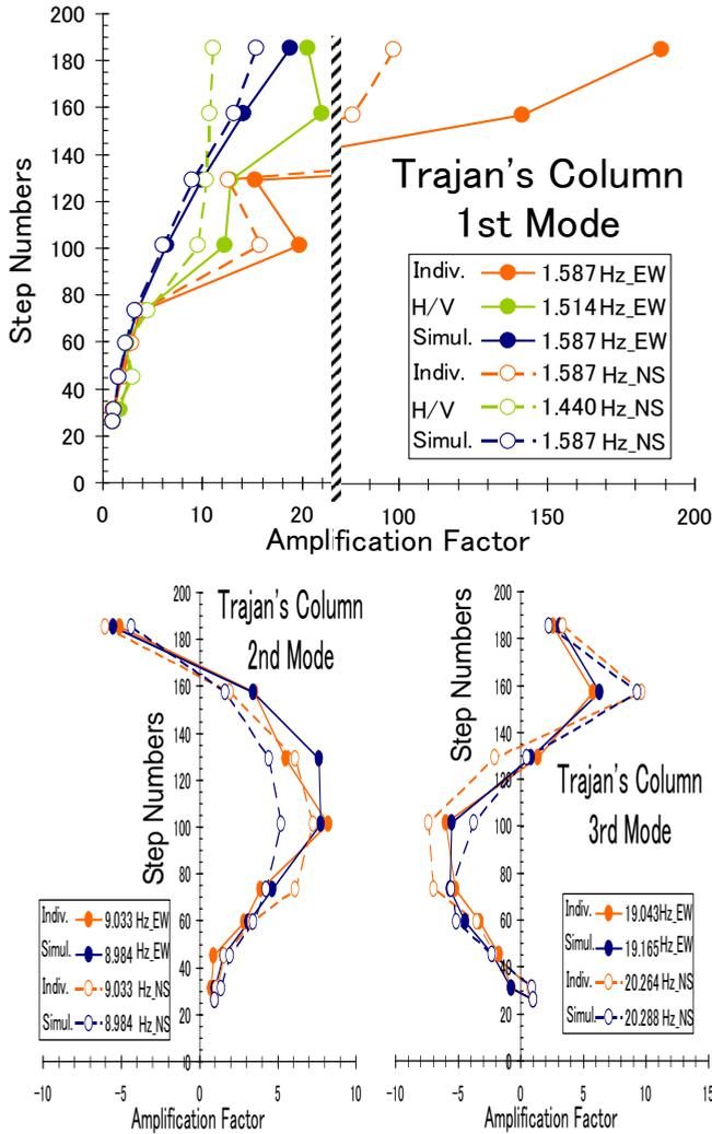
**Figure 6.** Comparison of the Shape of Modes of TC between Various Methods
