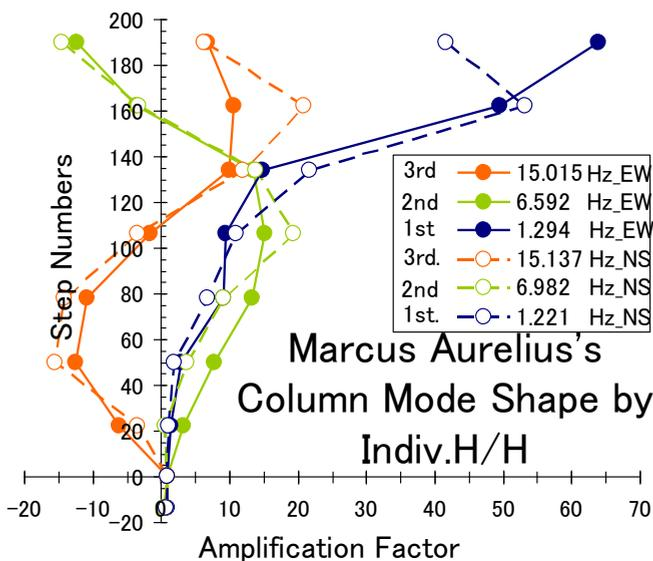
**Figure 9.** Mode Shape of AC estimated by Individual Measurements
