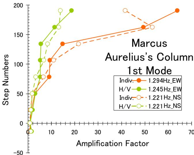
Figure 11. Comparison between First Mode Shapes of H/V and H/H of AC from Individual Measurements
