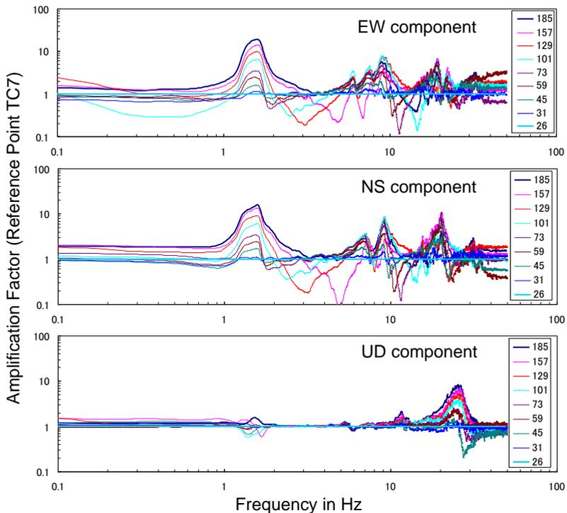
**Figure 3.** Amplification Spectra of TC estimated from Simultaneous Measurements
