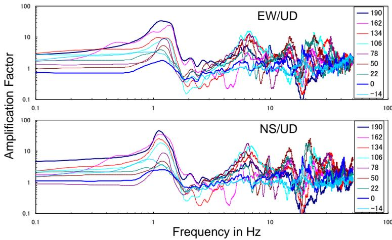
Figure 10. H/V Spectral Ratio at the sites of AC
