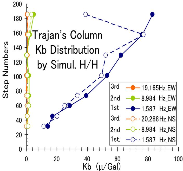
Figure 5. Kb-value of TC estimated from Simultaneous Measurement
