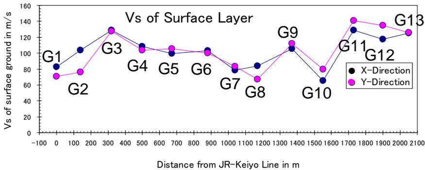
**Figure 10.** Distribution of  $V_s$  along the measuring line of Urayasu
