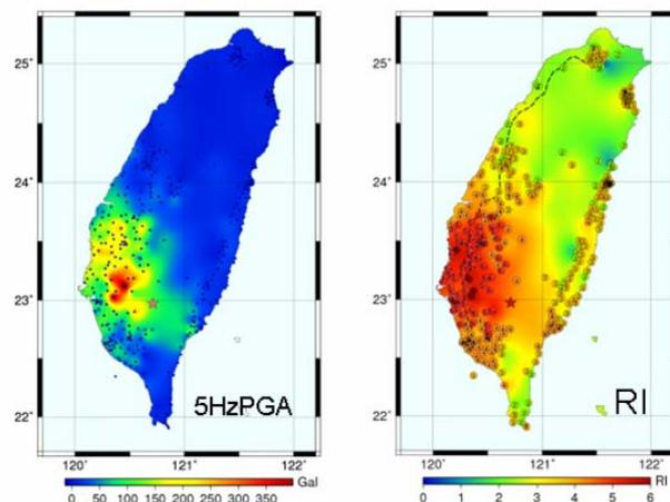
Figure 11 Distribution of Realtime Seismic Intensity and 5HzPGA of the 2010 Jiansian Earthquake, Taiwan
