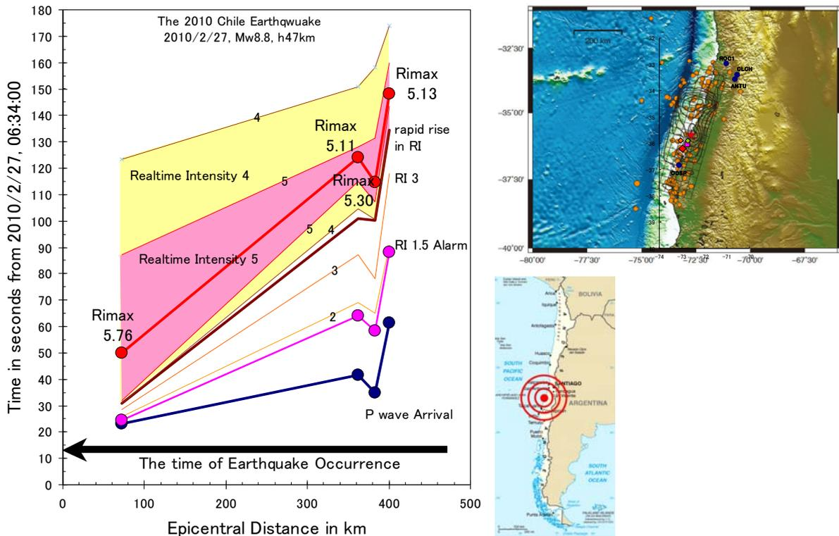
Figure 13 Simulation Result for the 2010 Chile Earthquake of Mw 8.8
