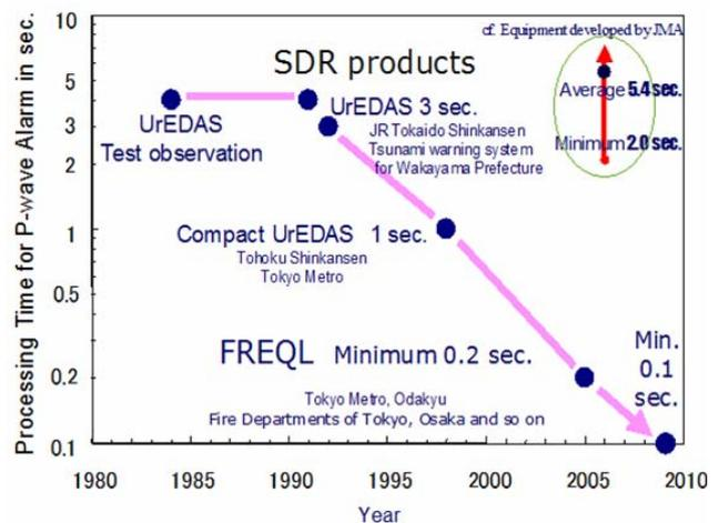
Figure 7 Processing Time of the EEW systems
