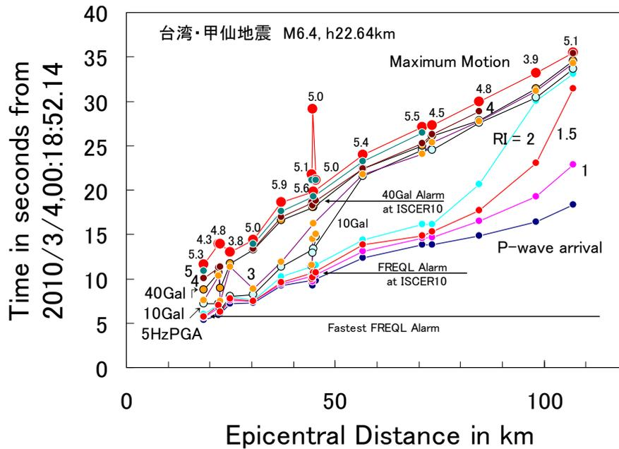
Figure 12 Simulation Result of FREQL Alarm for the Jiansian Earthquake
