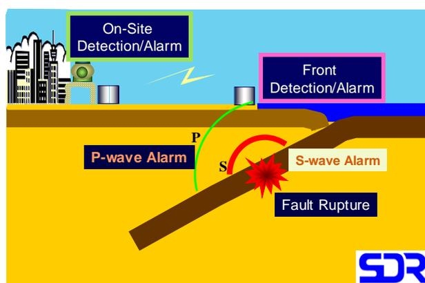
Figure 1 Concept of an EEW system
