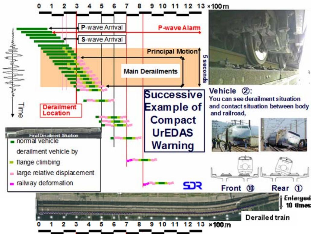
Figure 5 The Shinkansen Derailment during the 2004 Niigata-Ken Chuetsu Earthquake
