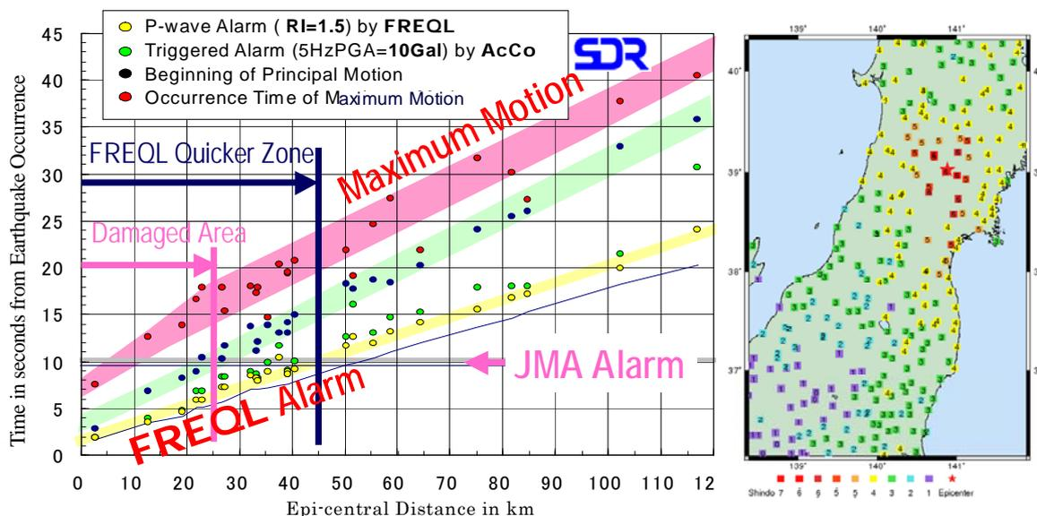
Figure 9 Comparison of EEW timing between *JMA* and *FREQ*L/*AcCo* for the 2008 Iwate-Miyagi-Nairiku Earthquake
