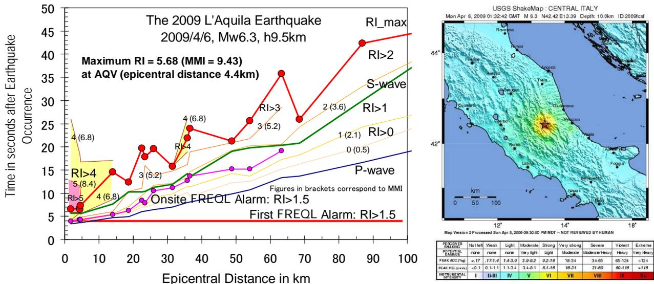
Figure 10. Timings of P wave arrival, FREQL warning, S-wave arrival and Maximum motion arrival: RI means Realtime Seismic Intensity; figures in brackets are corresponding to MMI.
