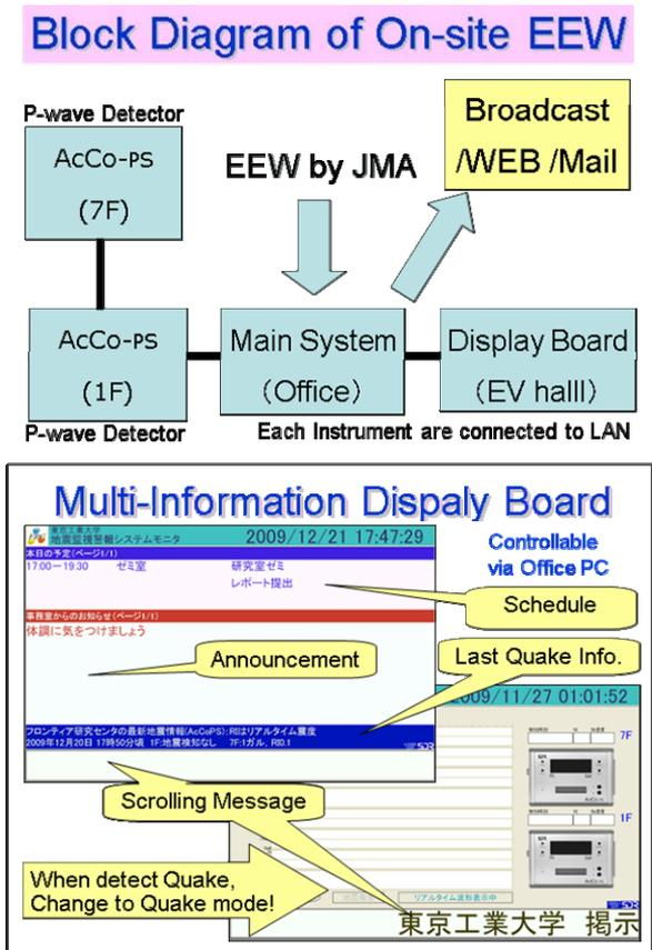
Figure 8 Block diagram of On-site EEW in Suzukakedai Campus of Tokyo Tech.
