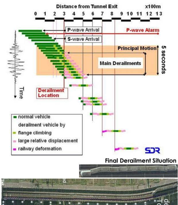
Fig.15 Estimated situation of the derailment
