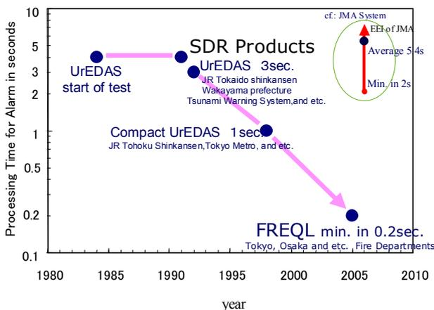
Fig.10 Change of processing time for EEW
