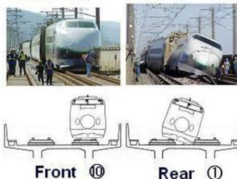
Fig.13 Detail of the derailment
