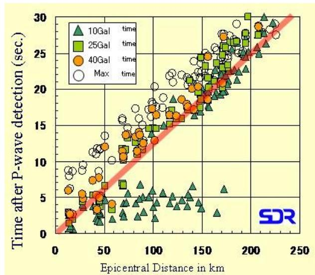
Fig.8 An example of alarm timings by simple triggers in case of the 2000 Tottoriken-Seibu Earthquake
