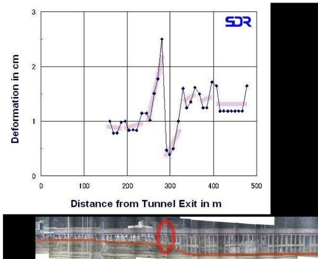
Fig.14 Performance of the deformation
