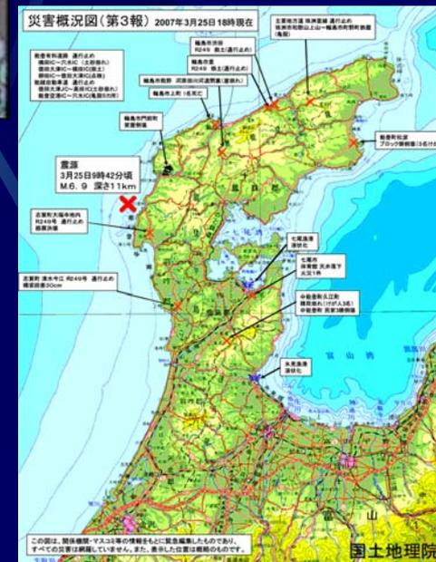
After the 2007 Noto-Hanto-Oki earthquake, during over three hours, Seismic Information (Location, Depth and Magnitude) was reported with wrong information. According to this wrong seismic information, no damage and no tsunami were assessed. But, unfortunately severe damage was reported in hours later. Quick response may be caused by the late result from this wrong information.
