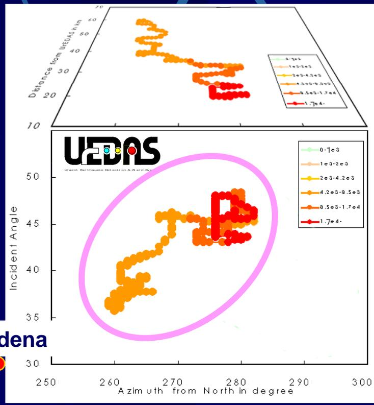
This is an example of rupture process tracing in realtime using the data of Pasadena UrEDAS station. The plane between back azimuth and incident angle is correspond to left upper cross-section. Rupture can be seen to go to surface from hypocenter.
