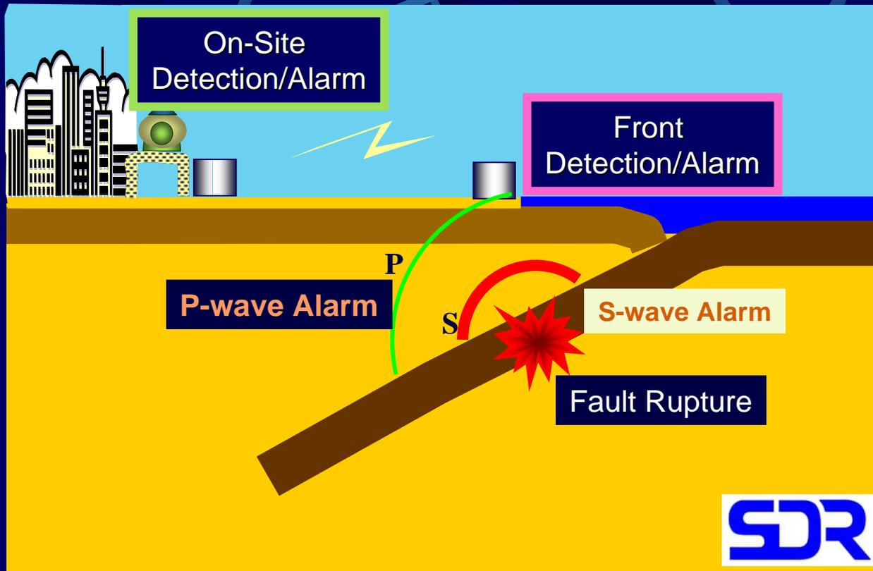
There are two kinds of the earthquake alarm. One is “On-site Alarm” which is the alarm based on the observation at the side of the objects to be warned. The other is “Front Alarm” which is the alarm based on the observation near the epicentral area to warn for the possible damaged area. For each, there are more two kinds of alarm. One is so-called “S-wave Alarm” or “Triggered Alarm”. And the other is “P-wave Alarm”.
