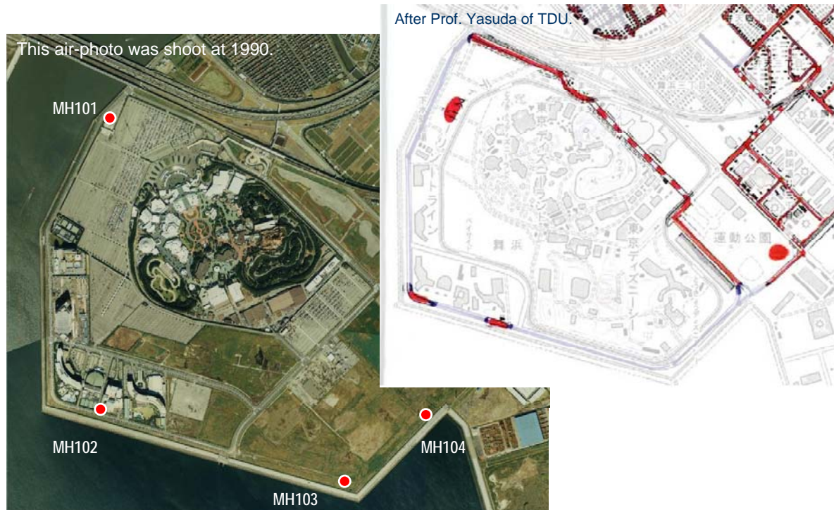
Figure 3.1. Measurement Point and Liquefaction Situation at Maihama Area
