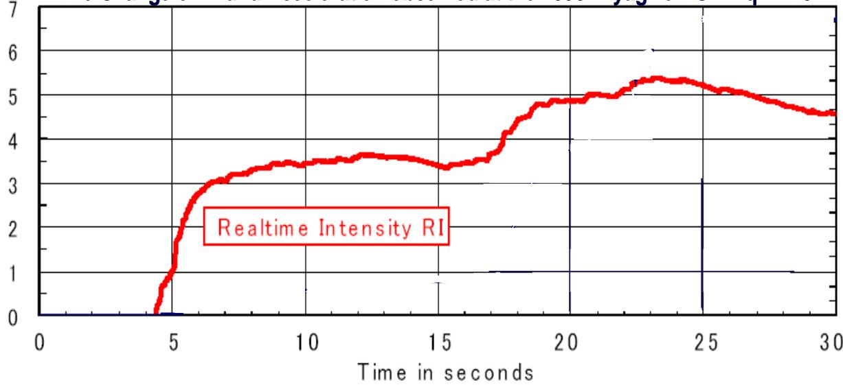
When P wave arrives, RI increases drastically. After initial P wave, RI keeps almost same value until the S wave arrival. After the arrival of S wave, it reaches to its maximum value. This value can be related on damage and Instrumental Seismic Intensity of JMA or other scales like MMI.
