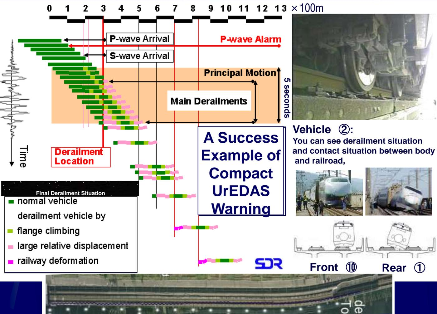
This shows the outline of the situation of the derailment. It seems that the derailed cars were running the large displacement section. The later the alarm reached, the more the number of derailed car, because of the risk of running the large displacement section. From the view point of this, the P wave alarm of Compact UrEDAS demonstrates the effectiveness for the derailment making not catastrophic.
