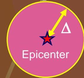
UrEDAS can issue an alarm based on the distribution of the past earthquake damage on magnitude to epicentral distance plane. This alarm is referred to as an M- $\Delta$  Alarm.
