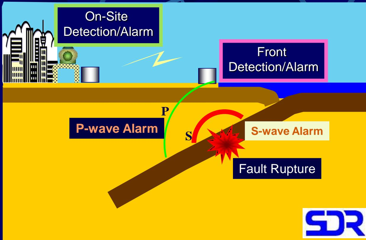
There are two kinds of the earthquake alarm. One is "On-site Alarm" which is the alarm based on the observation at the side of the objects to be warned. The other is "Front Alarm" which is the alarm based on the observation near the epicentral area to warn for the possible damaged area. Both alarm types described can make use of two different triggers, also called "alarms".
