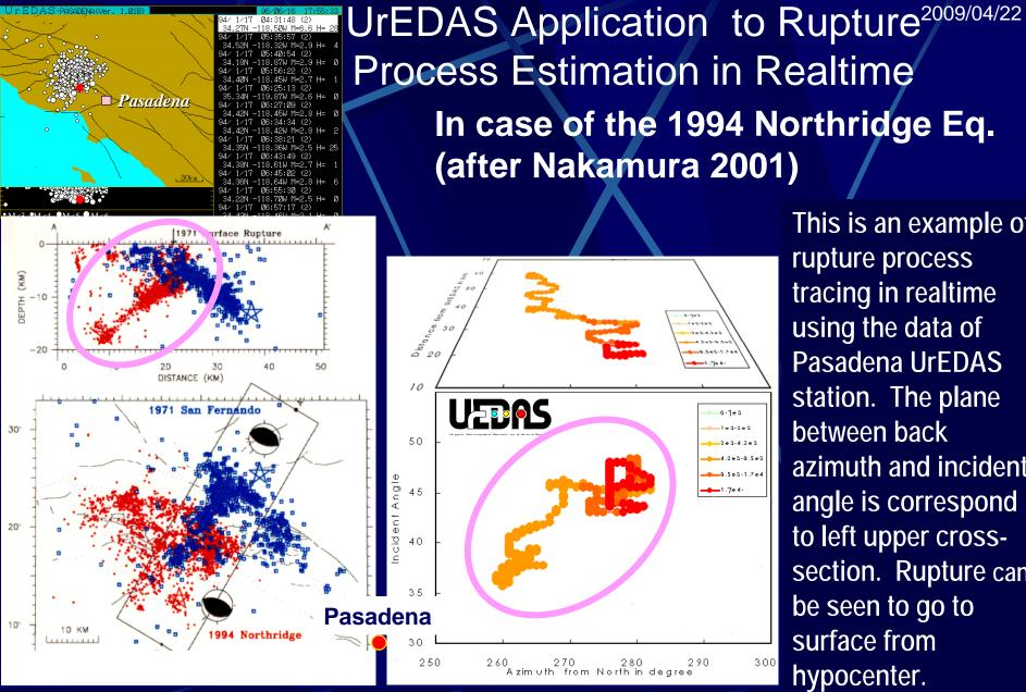
This is an example of rupture process tracing in realtime using the data of Pasadena UrEDAS station. The plane between back azimuth and incident angle is correspond to left upper crosssection. Rupture can be seen to go to surface from hypocenter.
