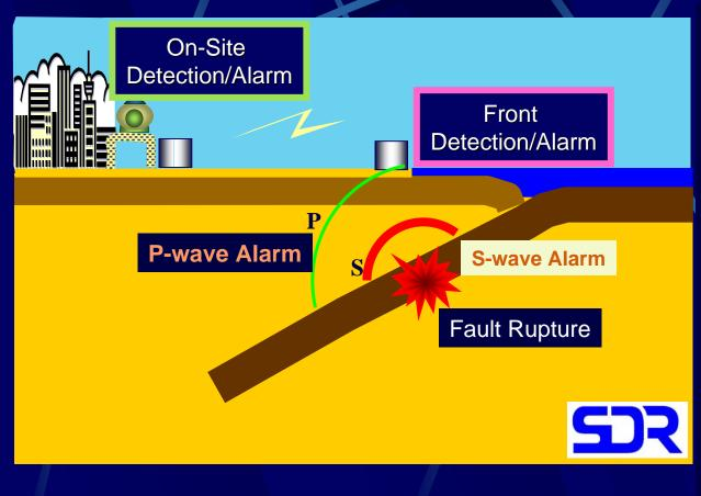
There are two kinds of the earthquake alarm. One is "On-site Alarm" which is the alarm based on the observation at the side of the objects to be warned. The other is "Front Alarm" which is the alarm based on the observation near the epicentral area to warn for the possible damaged area.
