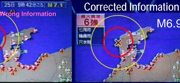
After the 2007 Noto-Hanto-Oki earthquake, during over three hours, Seismic Information (Location, Depth and Magnitude) was reported with wrong information. According to this wrong seismic information, no damage and no tsunami were assessed. But, unfortunately sever damage was reported in hours later. Quick response may be cased by the late result from this wrong information.
